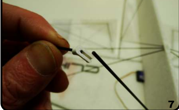
This "slot" is for the gear strut
