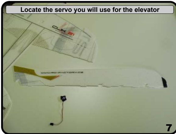
It will install into the cutout in the horizontal section
