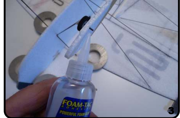
Make sure the wheel can spin and add a dab of glue
