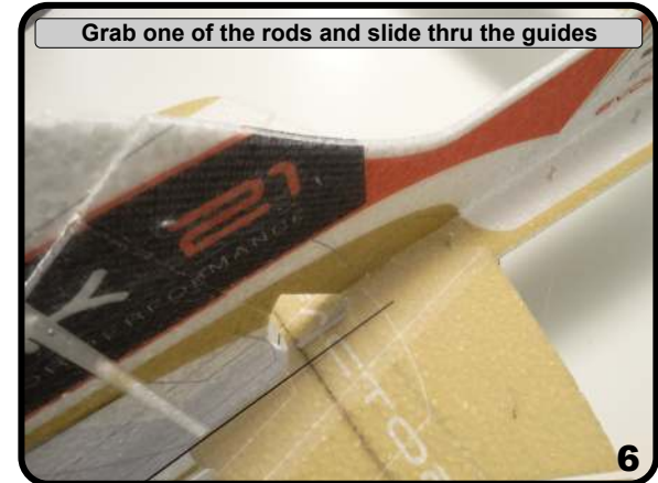
... and snap into the control horn hole with fingers
