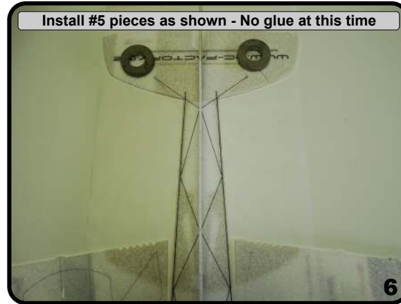
Make sure the fuselage is nice and straight
