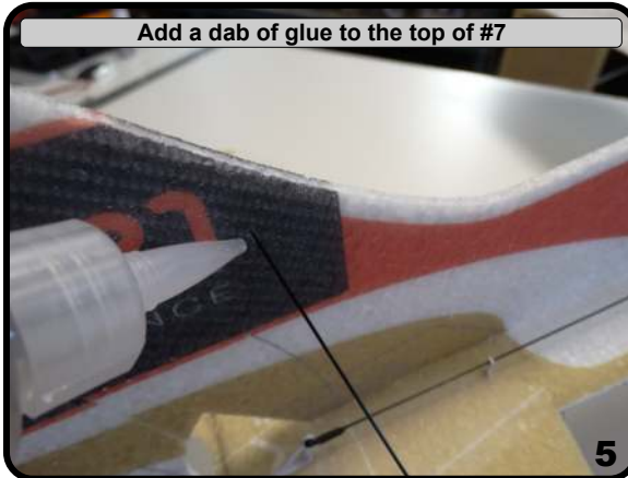
.. and adjust so that the rudder is nice and straight
