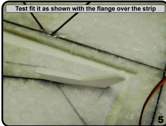
When happy with the fit remove and apply glue
