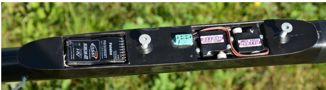
Servos and receiver installed in fuse
