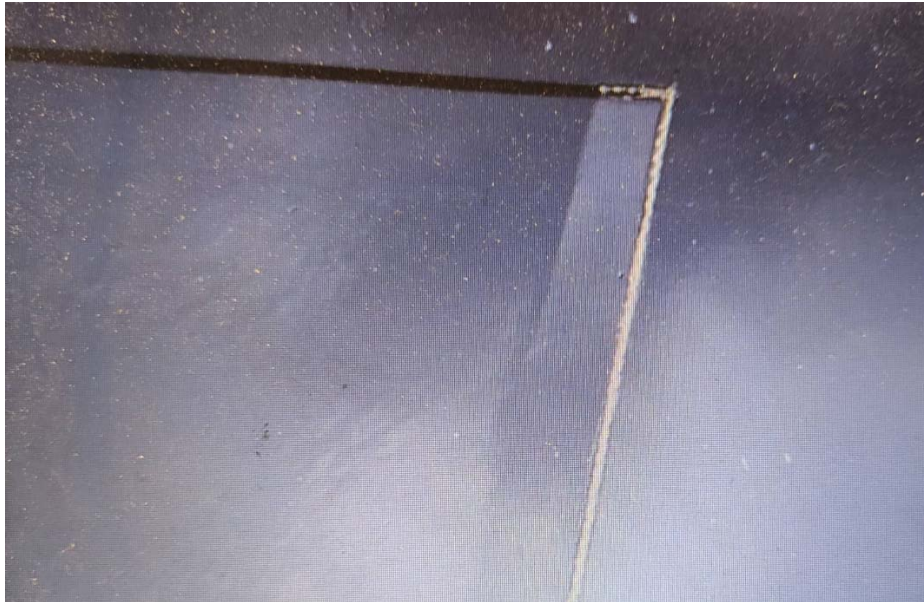
Damage to hingeline after too much movement (above 90 degrees) or flaps touching ground on landing
